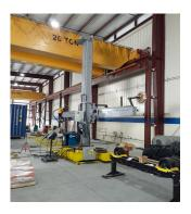
PRM's recent investments into the tank business include: a new 1000 Amp SubArc Welder which allows efficient, leak-free welds; tandem 20 ton overhead cranes, a complete new production building for tank fabrication, and CODEWARE software to ensure compliance with ASME VIII.
